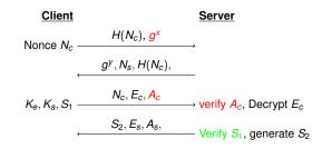
$$K_e = H_{g^{xy}}(N_s, H(N_c), 1), K_a = H_{g^{xy}}(N_s, H(N_c), 2)$$
